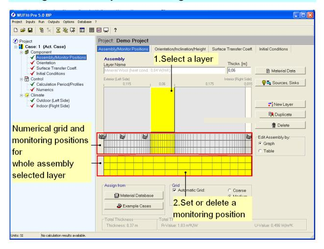
Select the layer where you like to insert a monitoring position. The numerical grid of the selected layer is then shown zoomed in the lower grid bar. Insert or remove a monitoring position by clicking on the desired element of the grid. Monitoring positions can only be set in the centre of a grid element and not between two elements.
