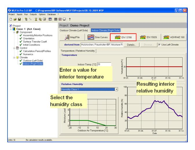
Normally the moisture load in residential buildings should be less than 4 g/m³ - this corresponds to humidity class 1 or 2. The values for humidity classes 3 and 4 are very high and should only be used if it has been established that in the investigated case the moisture load is indeed extremely high. They are not appropriate for normal residential buildings.
