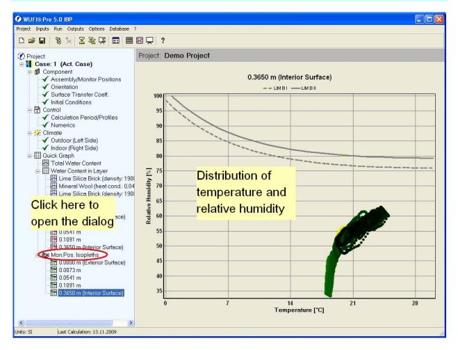
For each monitoring position, the quick graph "Mon.Pos Isopleths" plots the relative humidities at each time step against the simultaneous temperatures. This enables you to assess whether conditions of high temperature and high humidity occur at the same time which may create problems for some materials.
