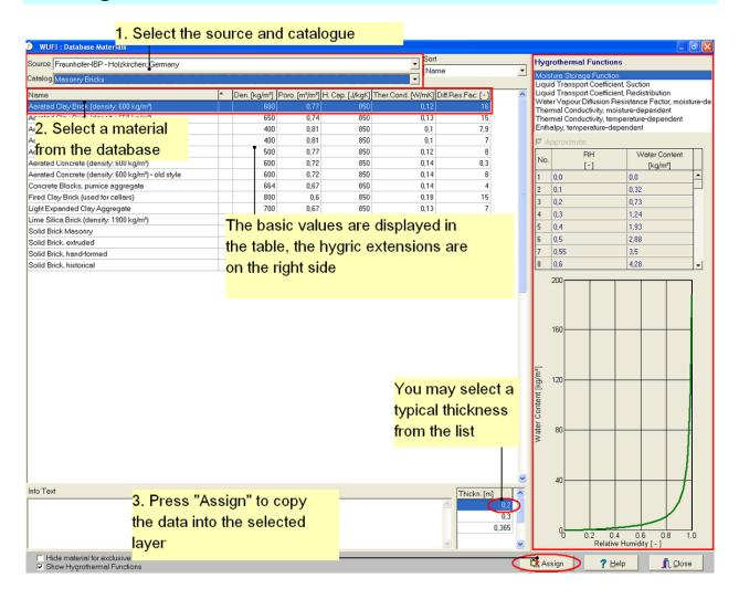
In this dialog you can select material data and assign them to the current layer. First select from the according drop-down lists the desired source and catalog. Here the source is "Institute for Building Physics in Holzkirchen - Germany" and the catalog is "Masonry Bricks". Then click on the desired material. The basic values of this material are listed in the table behind the material name. On the right side of the dialog the hygric extensions are shown.
