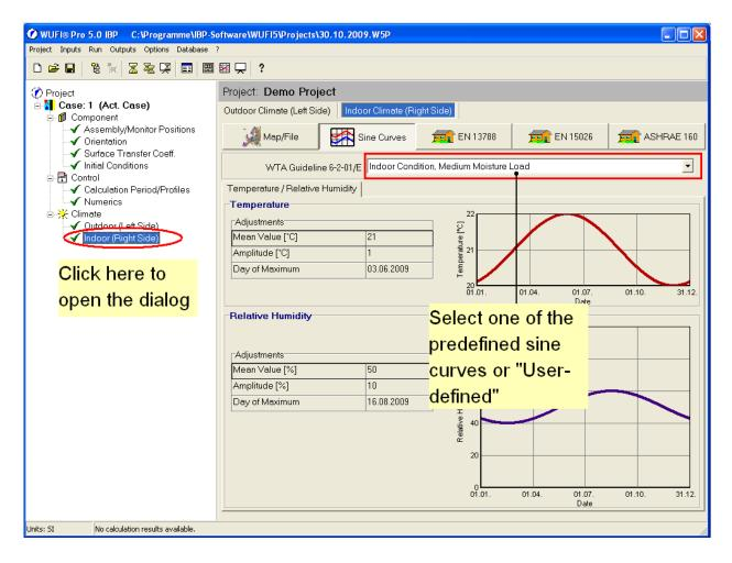
If you select "User-Defined Sine Curve Parameters" you can specify mean value, amplitude and day of maximum according to your wishes. You can also select a "constant" climate. For most cases the default values (medium moisture load, temperature 21°C with a 1 °C amplitude) are appropriate. So we use these settings the example case.
