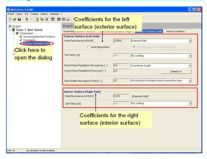
In the example case, "outer wall" conditions are assumed for the heat transfer. For the radiation absorptivity we select a light lime stone. As appropriate for a vertical wall a rain absorption of 70% is selected.
