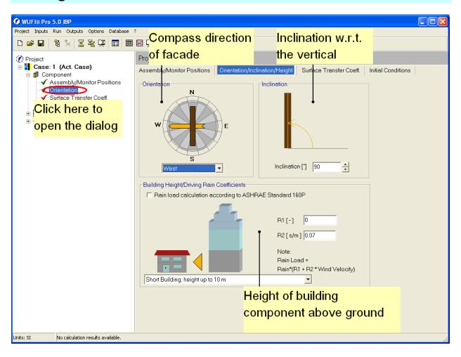
In the example case the choices are: orientation: west; inclination: 90°; height: "Short Building, height up to 33 ft".
