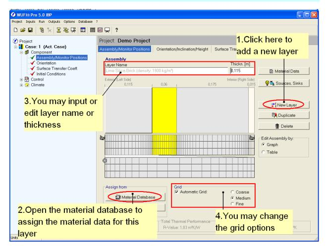
Use the button "New Layer" to create a new layer on the right side of the component. If needed, use the mouse to drag the layer to the desired location in the assembly. Then assign the appropriate material to the new layer using the button "Material Database" again.
