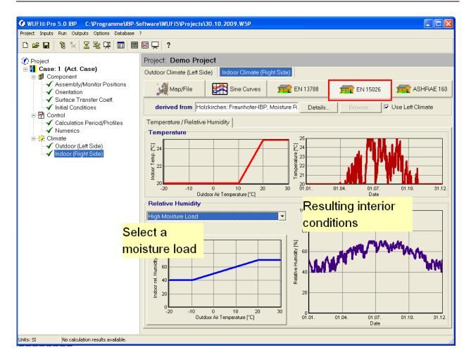
Specifically, the indoor temperature is kept at 20 °C for outdoor temperatures below 10°. For outdoor temperatures between 10 °C and 20 °C the indoor temperature varies in linear dependence of the outdoor temperature. For outdoor temperatures above 20 °C the indoor temperature is kept constant at 25 °C.
