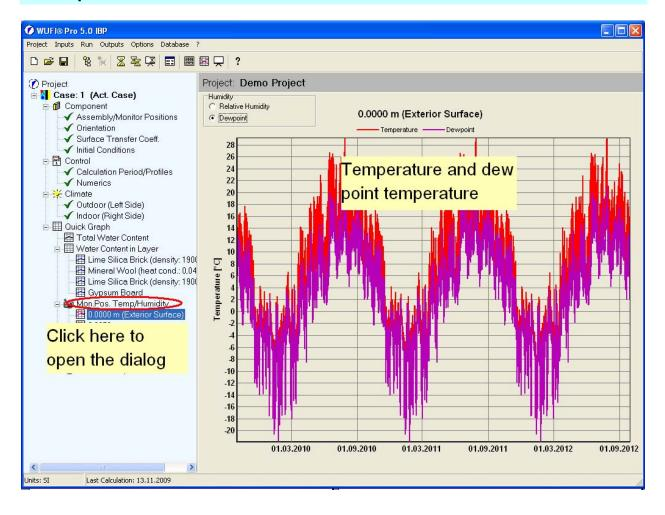
The diagram displaying the temperature and the dew point at the monitoring positions allows you to examine whether the temperature falls below the dew point at any time during the investigated period. This is the case when the red curve (temperature) is lower than the purple curve (dew point).
